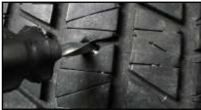
1. Injury no greater than 1/4" for passenger tires. Injury no greater than 3/8" for light truck/truck tires.
