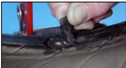
7. Deformed bead, exposed fabric or steel
