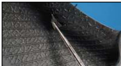
10. Tire damage from impacts
